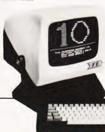
The Teleray Model 10, one of a three series range of micro-processor controlled VDU terminals.
